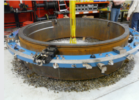
LDSF Split Frame for SG Replacement
