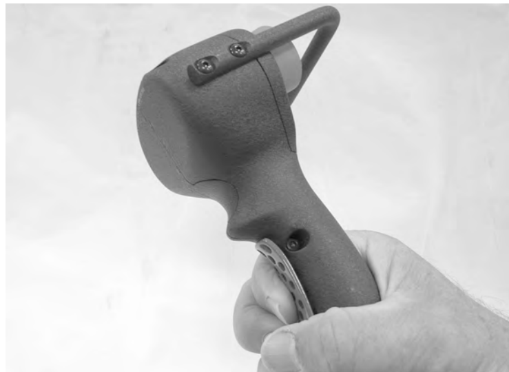
Figure 1-7. Squeeze the hold-to-run trigger to operate the motor. Releasing the trigger will stop the motor; to re-start, hold the trigger and press the Start button.
