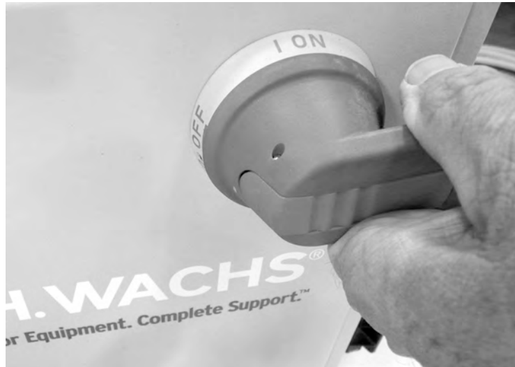
Figure 1-9. Turn the main power off when finished or when changing connections.
