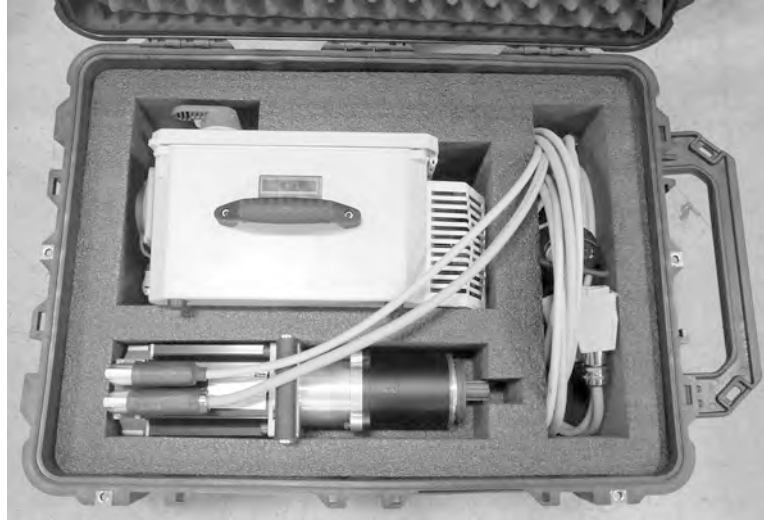
Figure 1-2. The drive system is provided in a custom storage/shipping case. Keep all components stored in the case when not in use.
