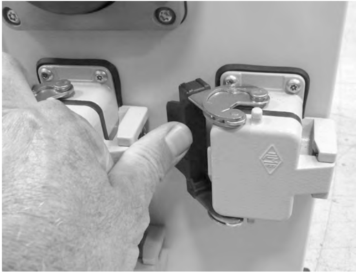
Figure 1-5. Press the tab as shown to unlock the connector cover.
