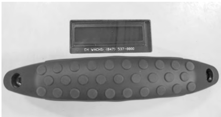
Figure 1-10. The LCD screen on top of the control cabinet displays error codes during operation.
