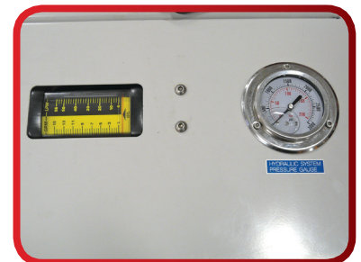
Pressure gauge and flow meter are easily viewed from the operator's position
