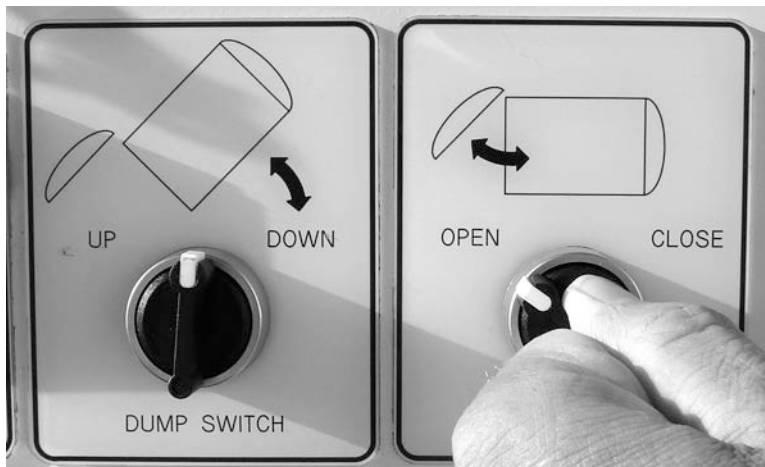
Figure 4-23. Turn the Latch Switch to the OPEN position and hold it until the door swings open.
