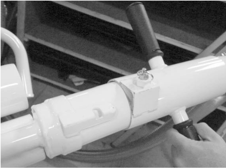
Figure 4-12. Slide the elbow onto the end of the wand. Align the locking pin in the elbow with the slot on the wand fitting.
