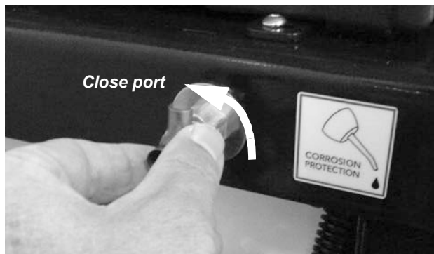
Figure 5-7. Close the blower lubrication port after spraying the lubricant.
