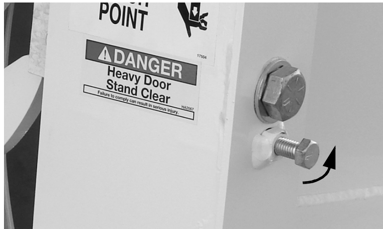
Figure 5-20. Turn the set screw counter-clockwise to loosen it.
