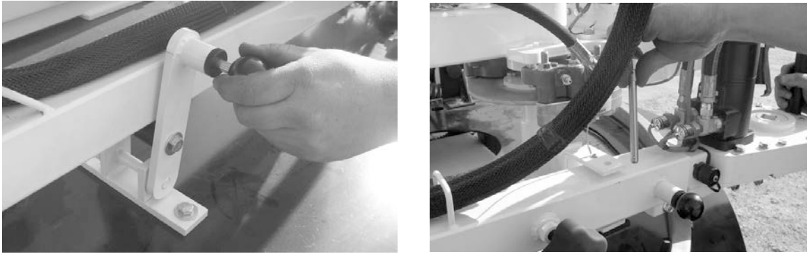
Figure 4-8. Release the two latches that secure the ERV-750 arm to the truck.
