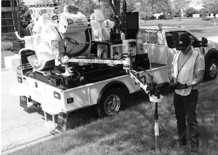
Figure 1-17. The ERV-750 valve operator extends on a telescoping swivel arm.
