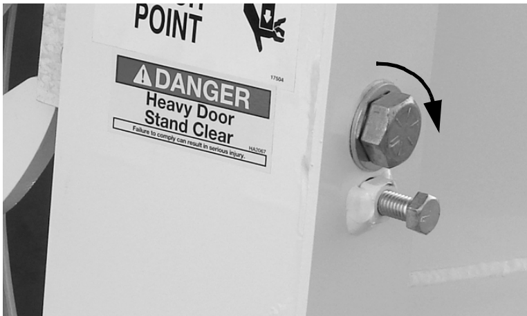
Figure 5-21. Turn the adjustment screw clockwise to tighten the latch.
