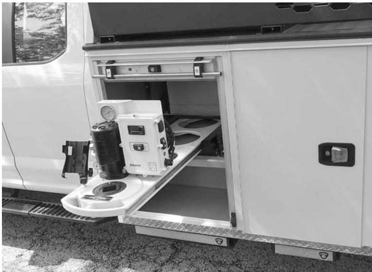
Figure 4-55. Loosen the lock knob on the side of the TM-7 slide rail, and pull the TM-7 out to the operating position as shown. Tighten the lock knob.
