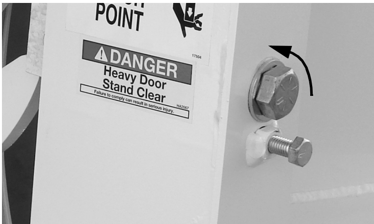
Figure 5-22. Turn the adjustment screw counter-clockwise to loosen the latch.
