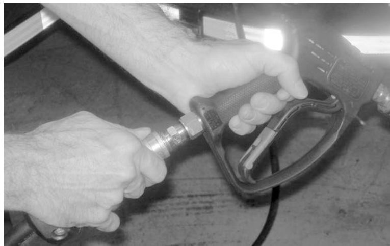
Figure 4-39. Attach the spray wand to the sprayer hose.
