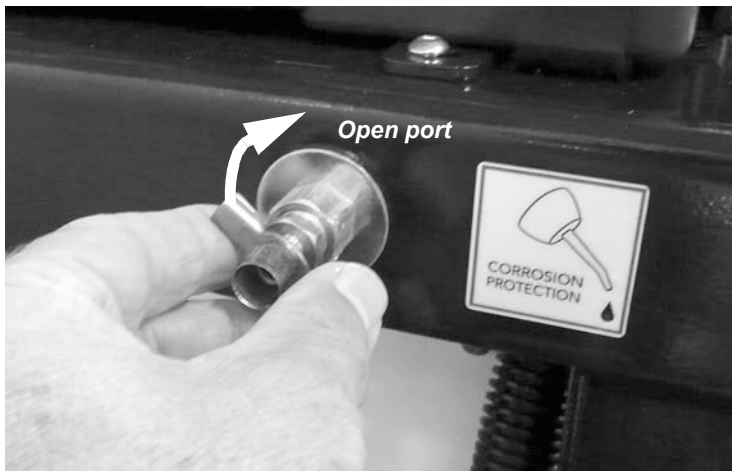
Figure 5-6. Open the blower lubrication port.
