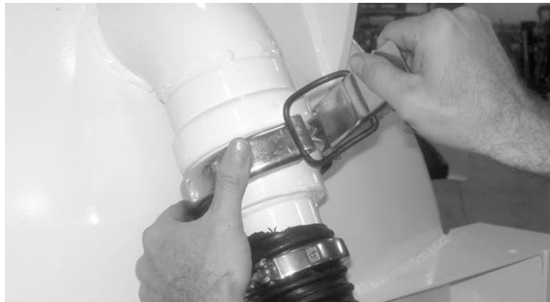
Figure 4-11. Insert the hose fitting into the inlet port and attach it with the locking collar.
