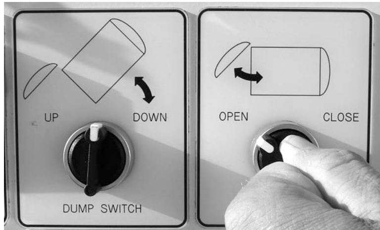
Figure 5-19. Turn the Latch Switch to the OPEN position and hold it until the latch fully opens.
