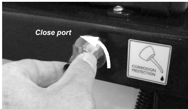
Figure 4-30. Close the blower lubrication port after spraying the lubricant.
