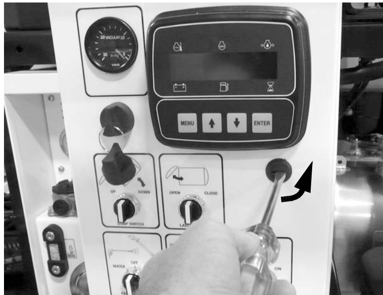
Figure 4-52. Use a screwdriver, coin, or the supplied engine key to open the control box and access the light bar control panel.
