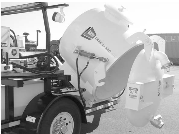
Figure 4-24. The tank door will swing open when the latches are released.
