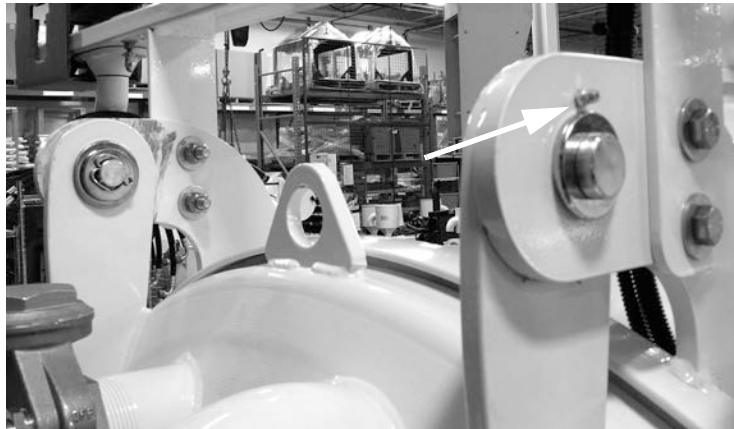
Figure 5-3. Apply grease to the tank door hinges at the 2 fittings (one each side).
