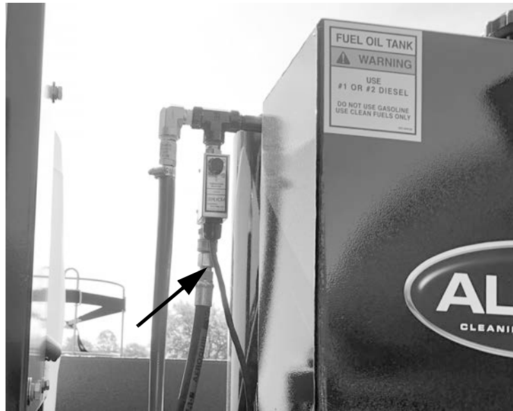
Figure 4-57. The photo shows the water heater outlet. To bypass the water heater, disconnect this hose at the location shown and connect it directly to the inlet hose (see previous figure).
