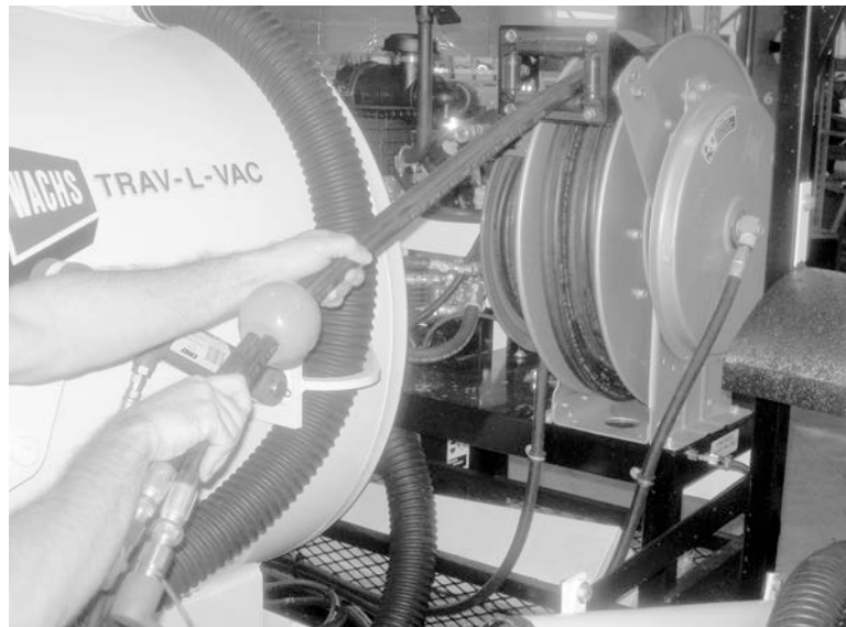
Figure 4-54. Pull the hydraulic hose pair off the hose reel to the work location.
