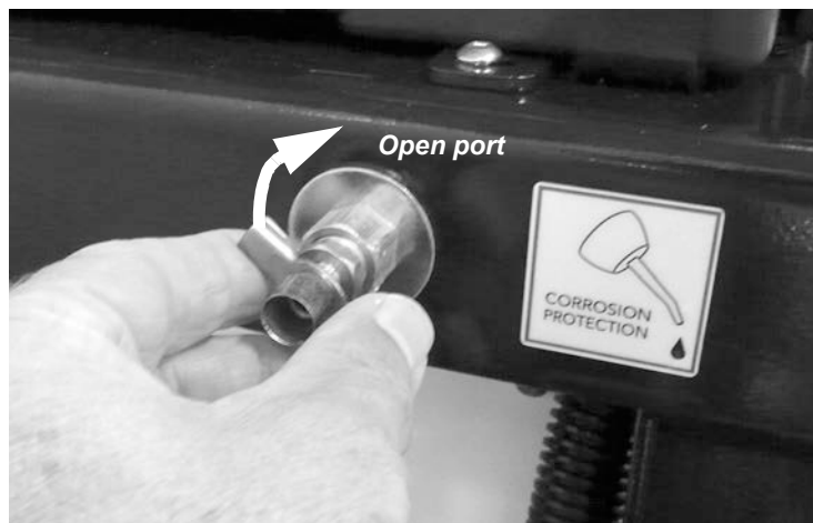
Figure 4-29. Open the blower lubrication port.
