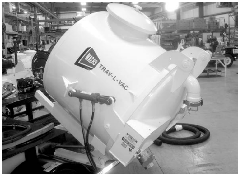
Figure 4-22. Tip the tank fully before opening the tank door.
