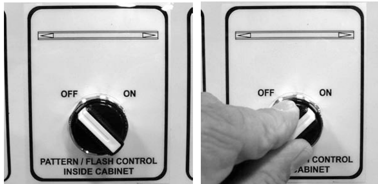
Figure 4-51. Turn the PATTERN/FLASH CONTROL switch ON to power the light bar.
