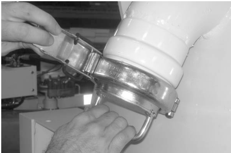
Figure 4-9. Pull the latch on the locking collar to release it and take it off the inlet port.
