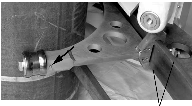
Figure 6-8. Grease the fitting for the clamping wheel and apply grease to the autoclamp rail.
