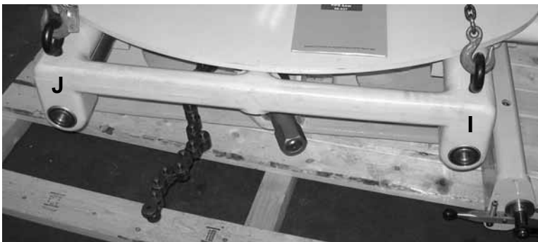
Figure 5-4. Eyebolts can be screwed into the threaded holes I and J in the end of the frame.
