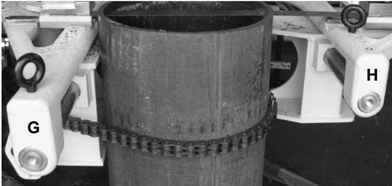
Figure 5-3. The eyebolts can be screwed into the threaded holes G and H on the end of the frame.
