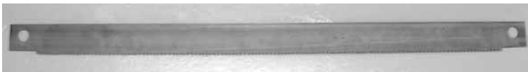
Figure 5-8. Goliath Guillotine blade. The mounting holes at each end are held by the dowel pins in the clamp blocks.
