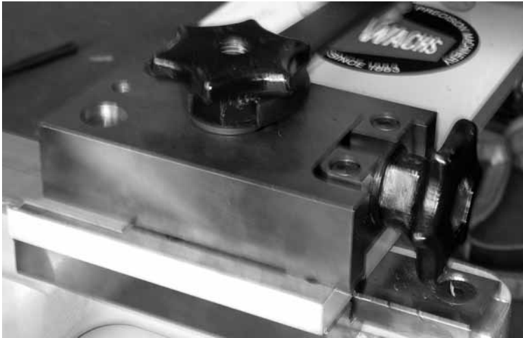
Figure 5-13. Tighten the clamp knob on both clamp blocks to secure the blade for cutting.
