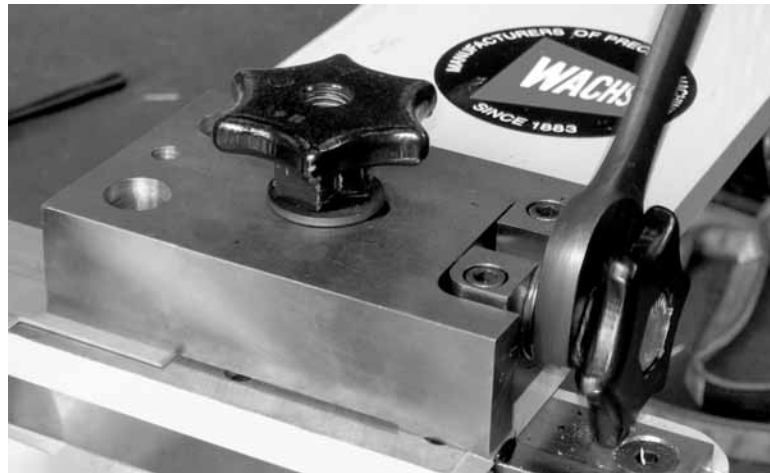
Figure 5-12. Tighten the tensioning knob to pull the saw blade tight.
