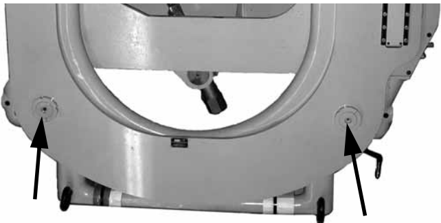
Figure 6-1. There are two grease fittings on the top of the saw bow.
