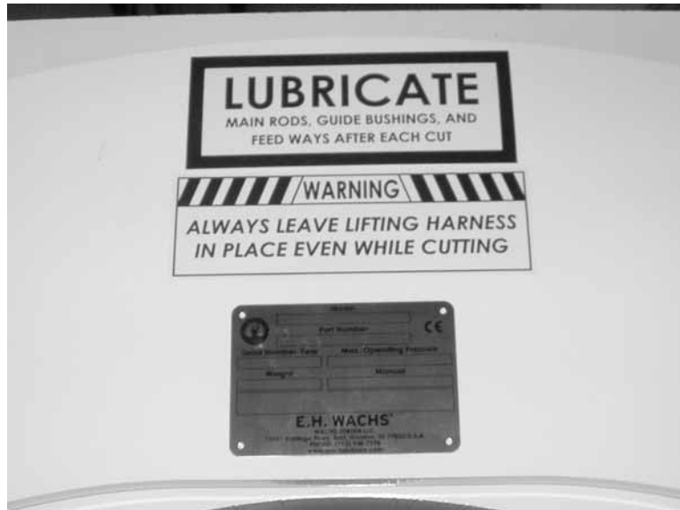
Figure 2-2. The Lubrication and Safety Harness labels are on the top of the saw bow, with the product plate.
