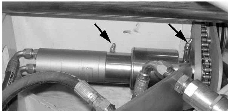
Figure 6-6. There are two grease fittings on the optional hydraulic autofeed motor.
