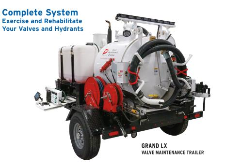
The Wachs Grand LX Valve Maintenance System has all the tools for water distribution preventative maintenance. Built for safe operation, a twoperson crew can find valves, wash out valve boxes, and safely exercise and rehabilitate valves up to 13 feet away with the ERV-750 valve exerciser. The included handheld computer with VITALS Software records the valve info and status for transfer back to headquarters.
