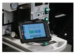
The ruggedized TC-100 handheld computer / wireless controller / datalogger provides intuitive remote exerciser control
