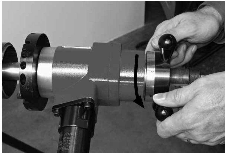
Figure 5-20. Retract the tooling after the operation is complete by turning the feed handle counter-clockwise.
