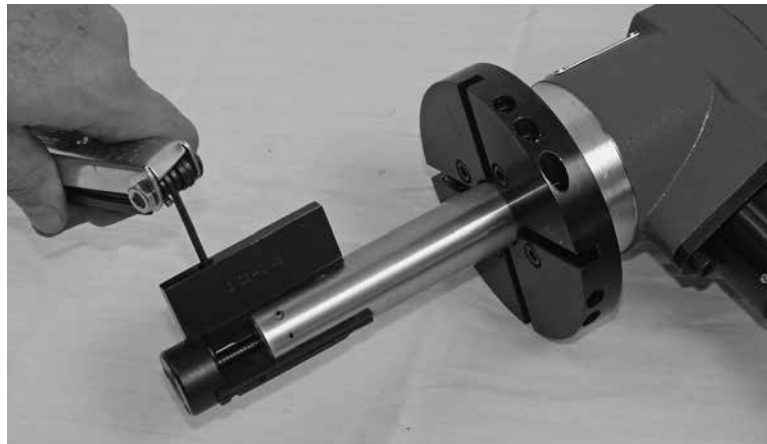
Figure 5-7. Attach the clamp legs to the mandrel and tighten the 2 screws in each leg.
