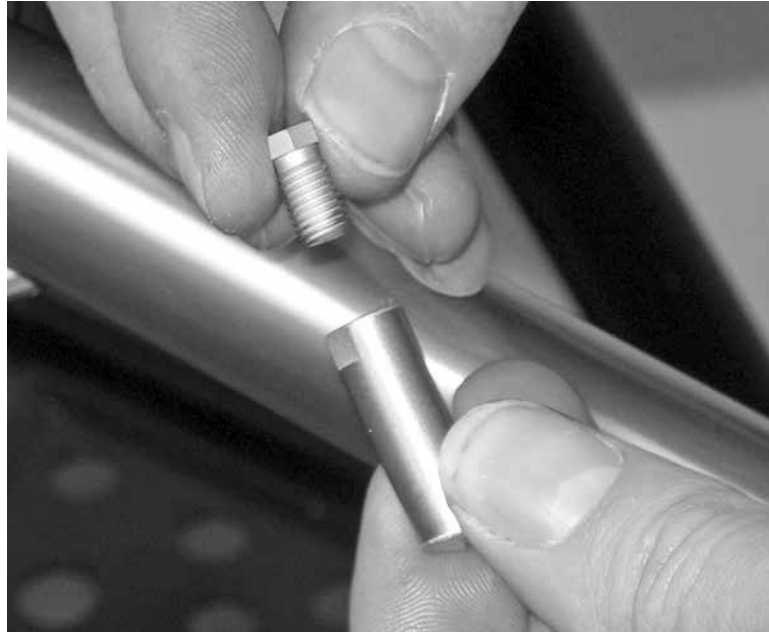
Figure 5-33. Attach the leg adjustment screw to the adjustable leg.
