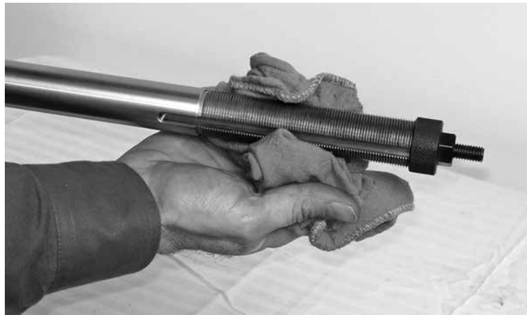
Figure 5-1. When cleaning the mandrel, inspect the threads for damage.
