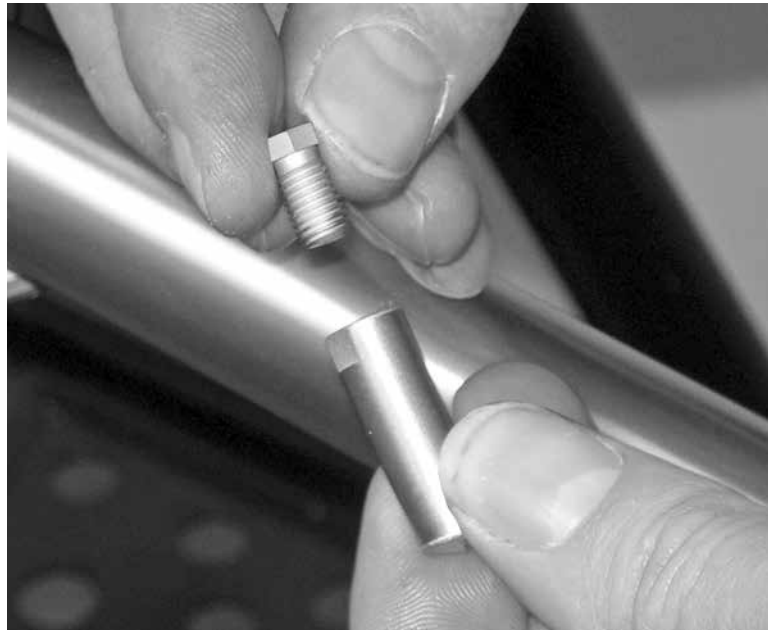
Figure 5-8. Attach the leg adjustment screw to the adjustable leg and screw it in fully.
