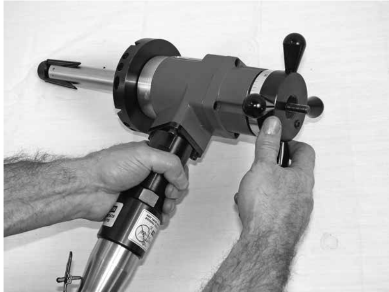
Figure 5-3. Turn the feed handle to thread the mandrel into the machine body
