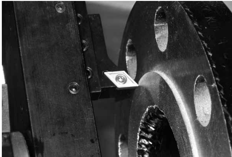
Figure 5-38. Position the single point cutting tool with the cutting surface in the direction of rotation.
