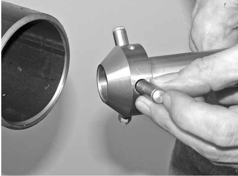
Figure 5-9. Insert the legs into the independent fitting mandrel.
