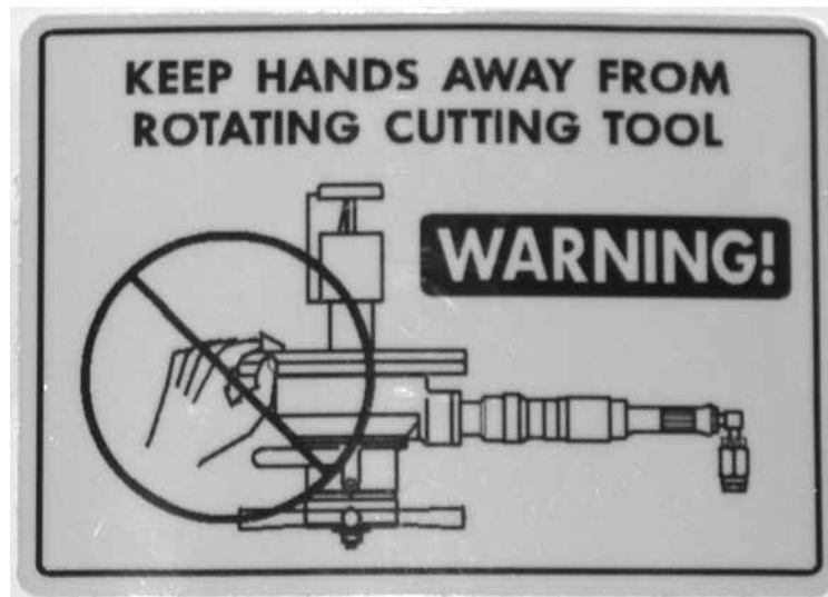
Figure 2-2. The Warning sticker is on the SDB 103. Do not put your hands near the rotating head while the machine is running. (Part number 66-147-00.)
