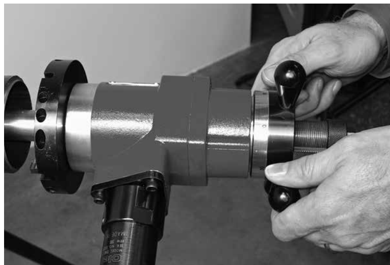
Figure 5-25. Turn the feed handle counter-clockwise as shown to retract the tool bits.
