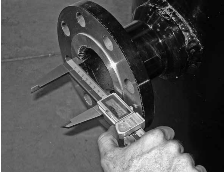
Figure 5-32. Measure the I.D. of the flange.
