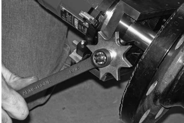
Figure 5-37. Turn the starwheel counter-clockwise to retract the tool slide past the O.D. of the flange.
