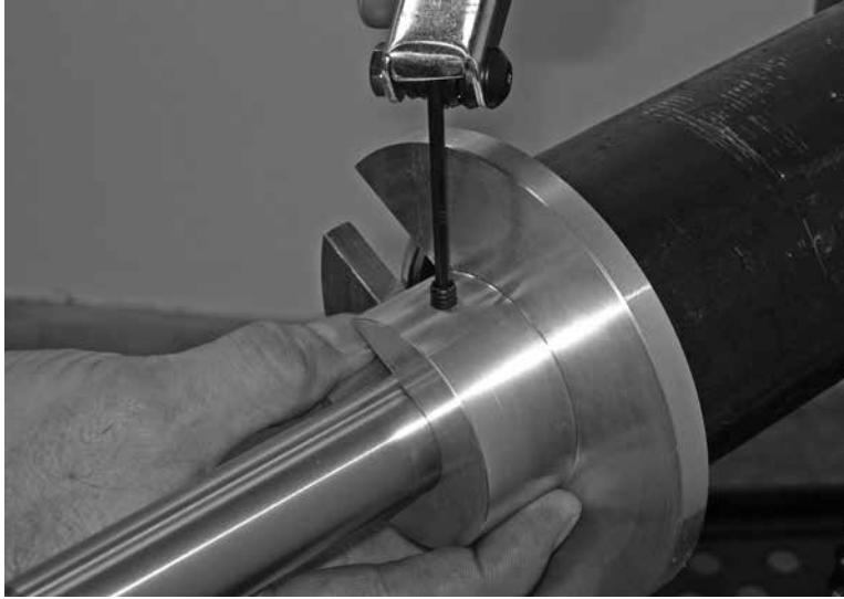
Figure 5-14. Tighten both set screws in the squaring plate to secure and center it to the mandrel.
