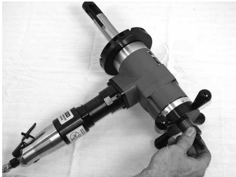
Figure 5-4. Tighten the collar nut with finger pressure to captivate the draw bar nut on the mandrel.
