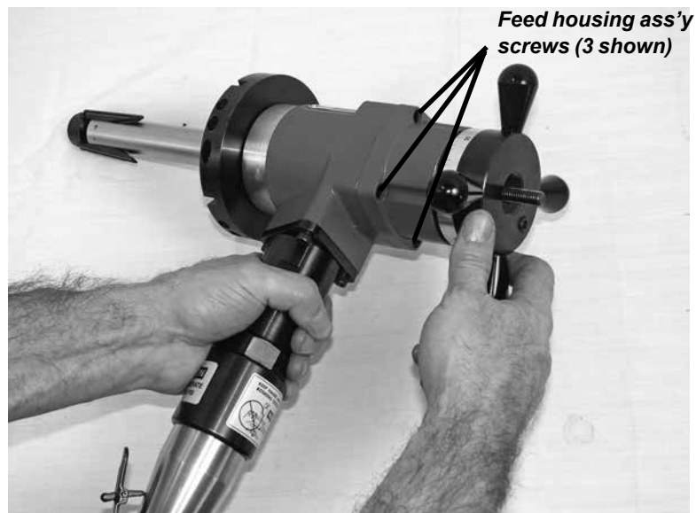
Figure 6-1. Remove the 4 screws attaching the feed housing assembly.
