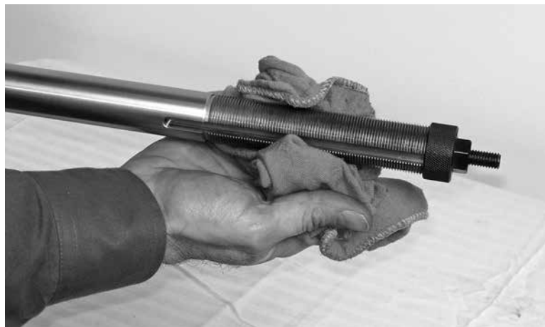
Figure 6-3. When cleaning the mandrel, inspect the threads for damage.
