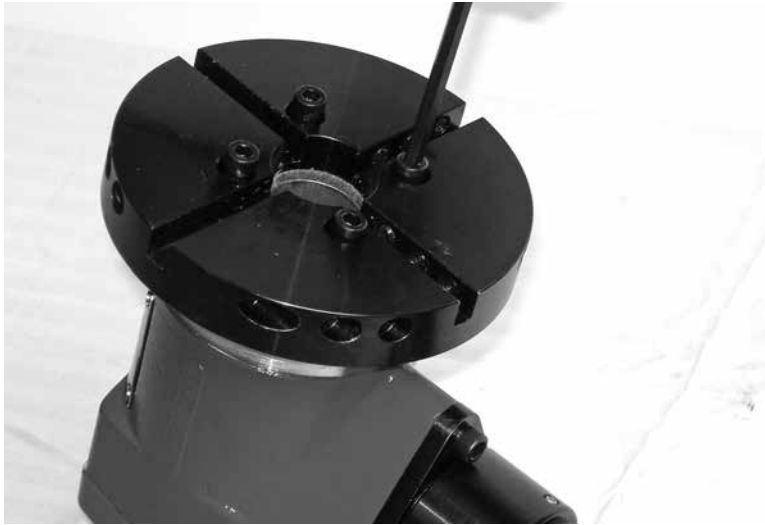
Figure 5-29. Remove the rotating head screws using a 3/16" hex wrench.
