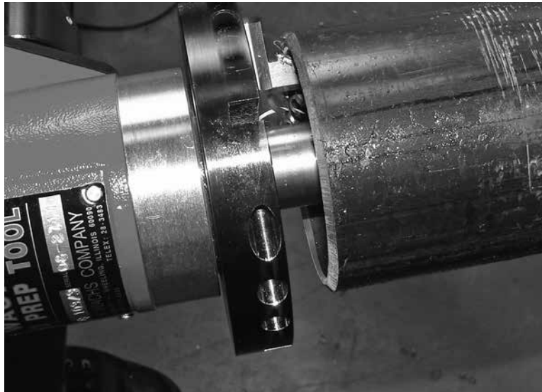
Figure 5-23. Run the machine until the desired counterbore is cut.
