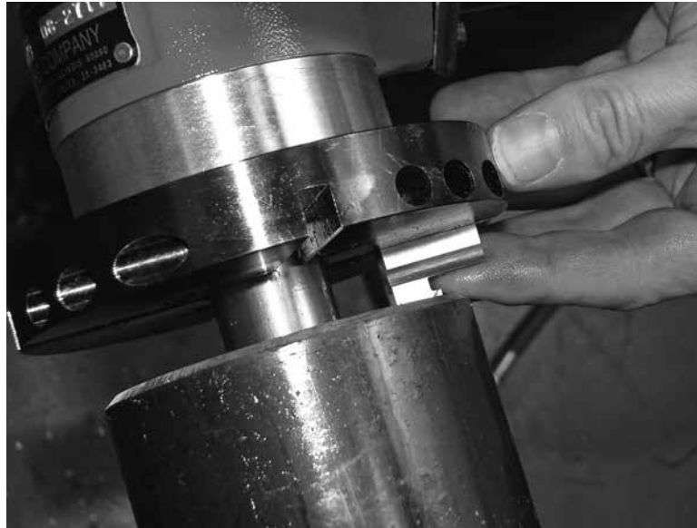
Figure 5-21. Insert the counterbore tool but do not snug the tool bit wedge screws.
