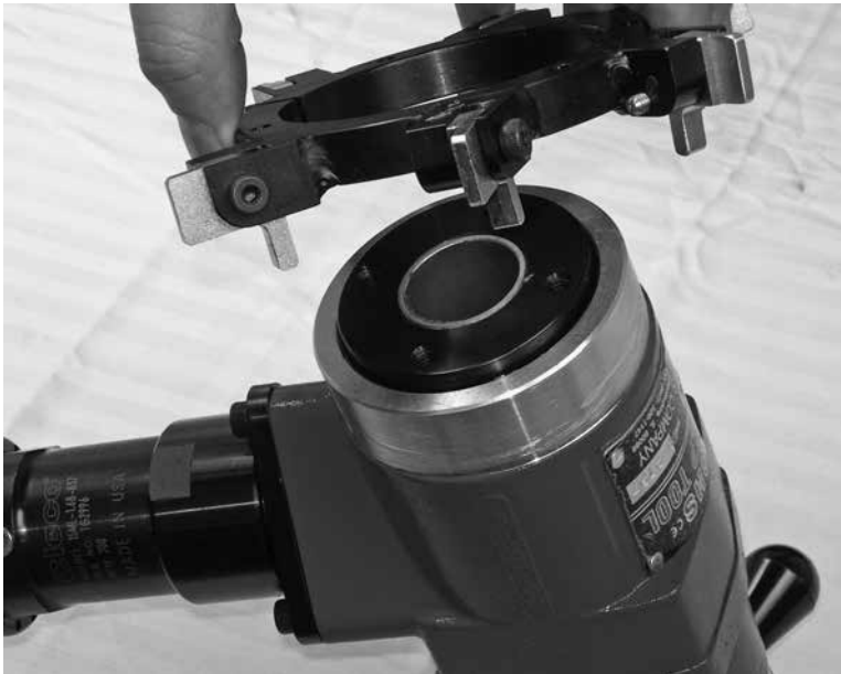
Figure 5-30. The trip collar locking screw should be as close to the air motor housing as possible.
