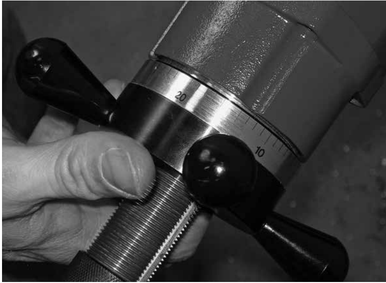
Figure 5-26. The calibrated feed handle is graduated in 1/1000" increments.
