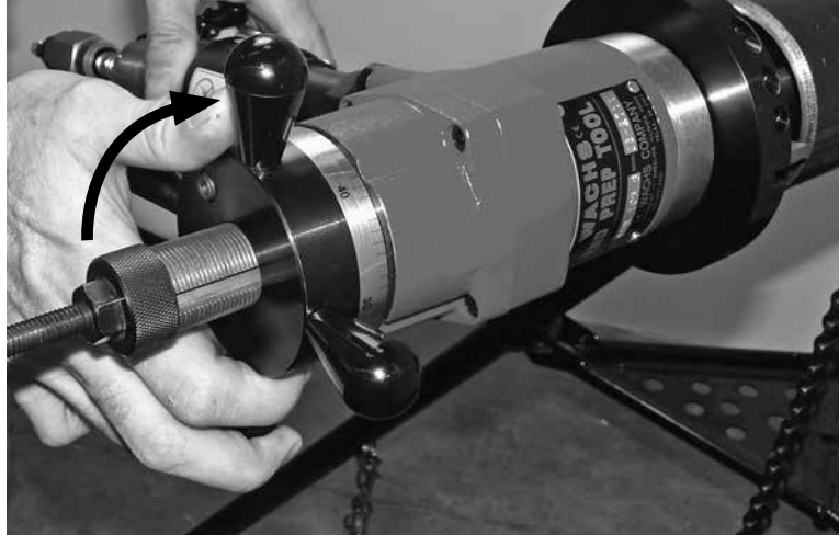
Figure 5-19. To face the pipe, turn the feed handle clockwise.
