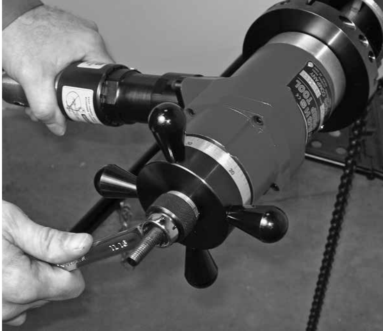
Figure 5-11. Hold the machine in place and tighten the drawbar nut.
