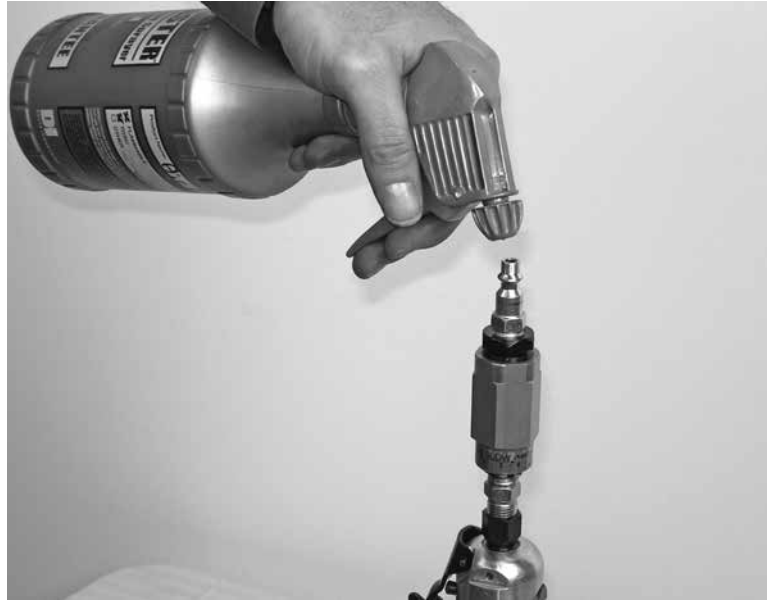
Figure 6-2. Apply air motor oil to the air motor daily.
