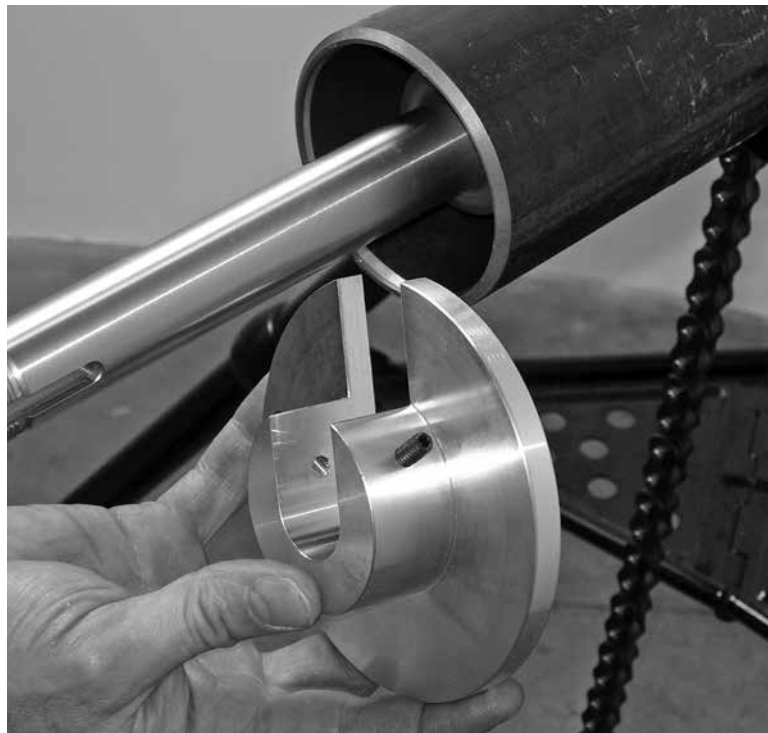
Figure 5-13. Put the squaring plate onto the mandrel.
