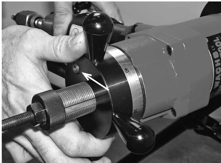
Figure 5-41. Snug the feed handle set screw to keep the machine from moving radially when flange facing.
