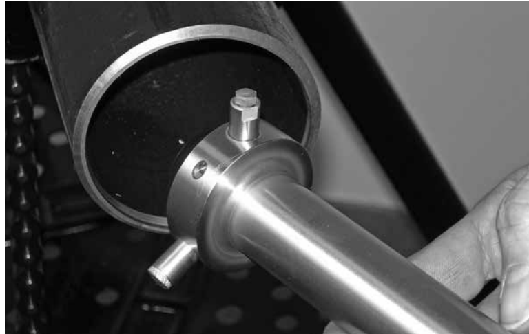
Figure 5-12. Insert the mandrel into the pipe.
