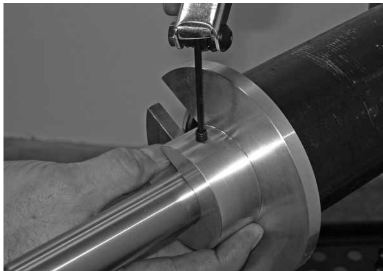
Figure 5-34. The squaring plate automatically squares the FF 206 to the pipe face.
