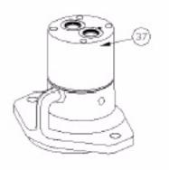
STN-65132 Motor assembly used on sump pumps with serial numbers 600 and above. This motor can only be purchased as an assembly; individual parts are not available.
