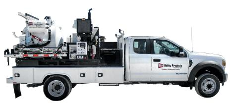
Wachs has partnered with Knapheide to improve the efficiency of the Valve Maintenance Skid (VMS) through the design of a specialized service body; this unique solution optimizes vehicle storage and equipment layout, making for an efficient workflow.
