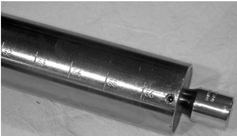
Figure 1-3. The EICC drive tube is graduated in inches to allow for quick, accurate setup. The numbers indicate how far the cut line is below the surface of the wellhead.
