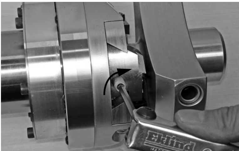
Figure 3-23. Retract the tool slide one complete revolution clockwise from its innermost position.
