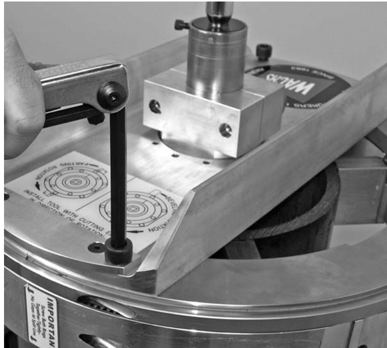
Figure 3-27. Mount the bridge to the LCSF as shown.
