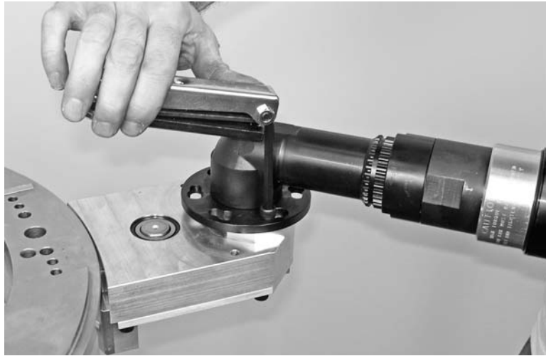
Figure 3-4. Secure the air motor using the mounting screws as shown.
