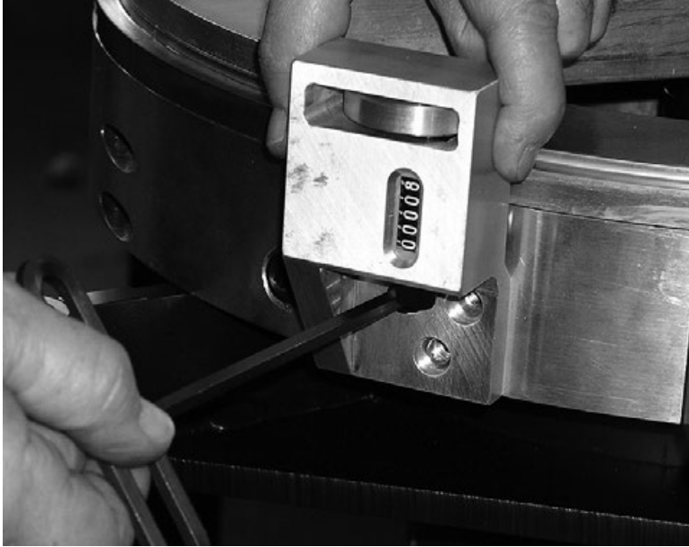
Figure 3-29. This photo shows the counter being mounted to the LCSF.
