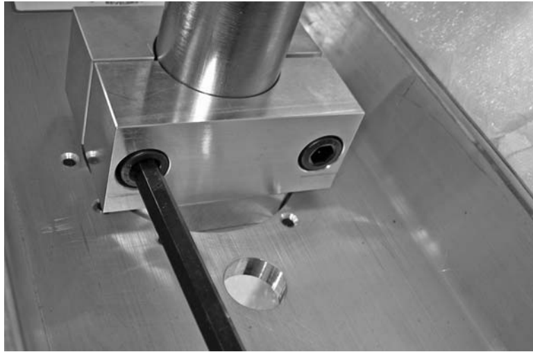
Figure 3-9. Align the bridge collar at the desired depth mark, and then tighten the bridge collar clamp screws.
