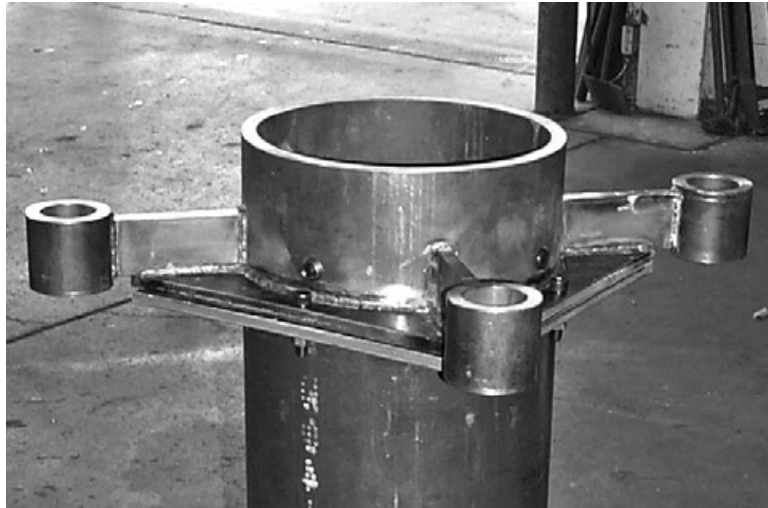
Figure 1-9. The wellhead adapter holds the LCSF in the proper vertical position while the EICC is centered inside the production casing.
