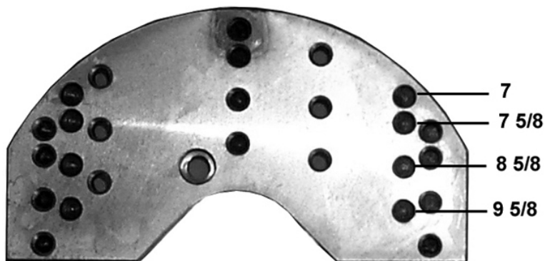
Figure 3-12. The standard tool slide mounting locations are shown above. Insert the mounting dowel pins into the holes corresponding to the production casing size (in inches) you are cutting.
