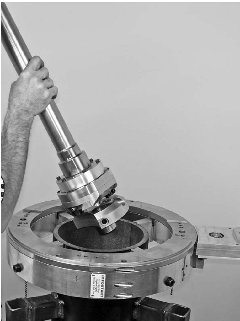
Figure 3-26. Insert the internal cutting module into the casing.
