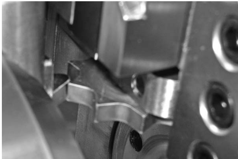
Figure 3-18. Verify that the trip pin contacts the star-wheel as shown.
