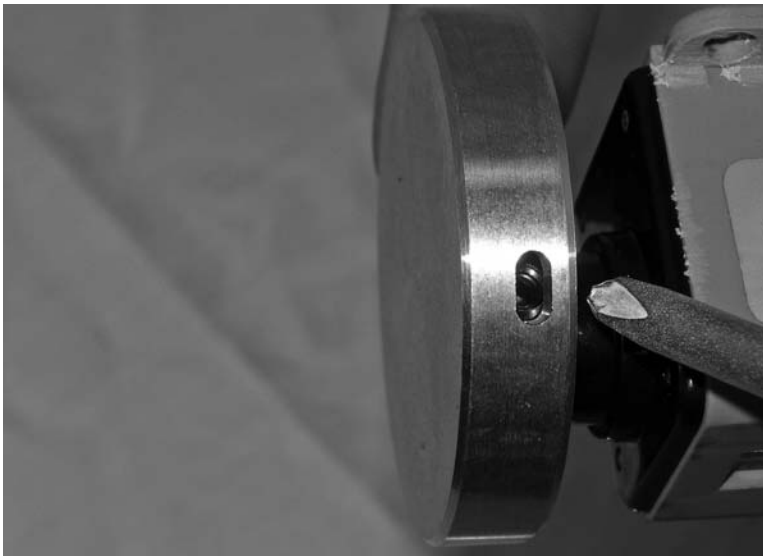
Figure 4-3. The hex screw is accessible through the counter wheel notch.
