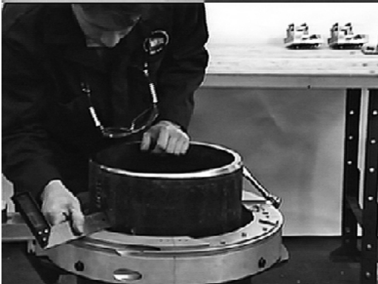
Figure 3-2. Square the LCSF on the casing before proceeding.
