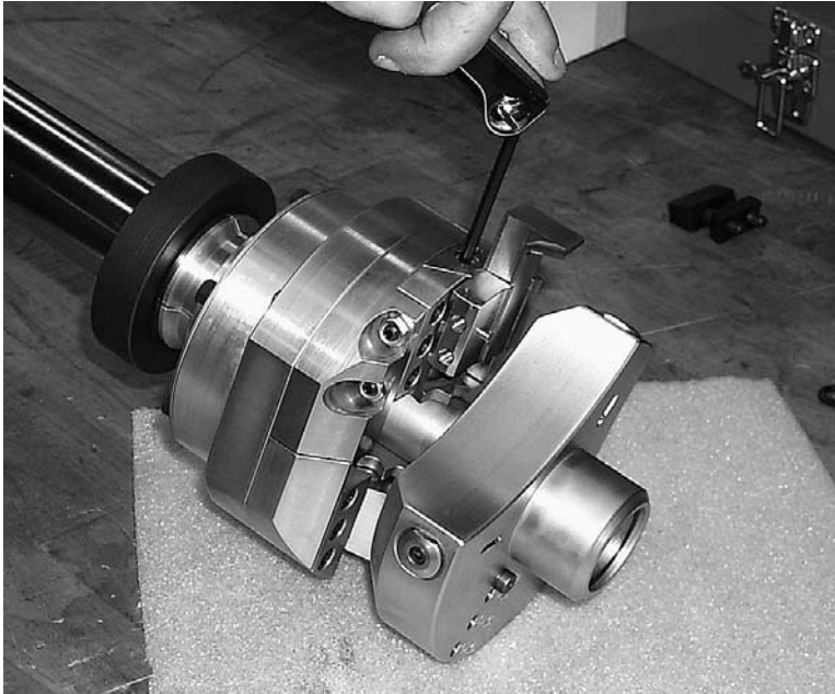
Figure 3-37. Adjust the tool slide as noted.
