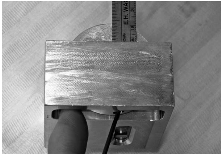
Figure 4-5. Use a scale to accurately adjust the counter wheel.
