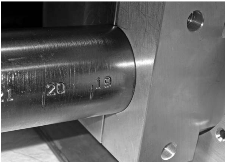
Figure 3-8. Use the depth marks on the drive tube to align the internal cutting attachment.
