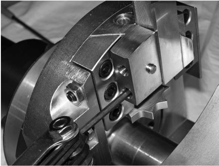
Figure 3-22. Tighten the tool slide screws to secure the tooling.
