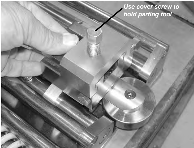
Figure 3-39. Slide the tool cover onto the tool holder and position it flush at the front.
