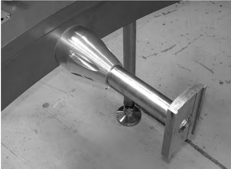
Figure 3-20. Insert the clamp leg through the cone spacer and turn the adjustment screw to thread it in.
