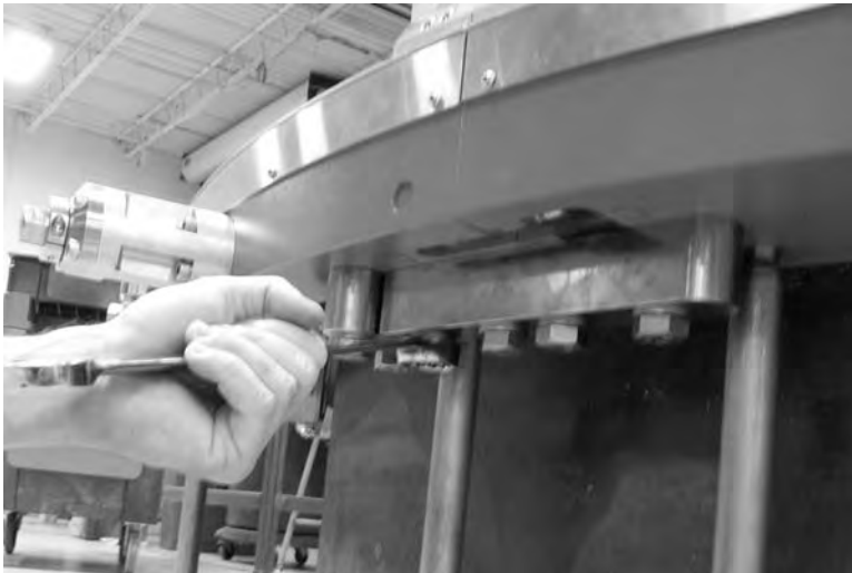
Figure 3-14. Install the support block at each split line and tighten the 4 screws.
