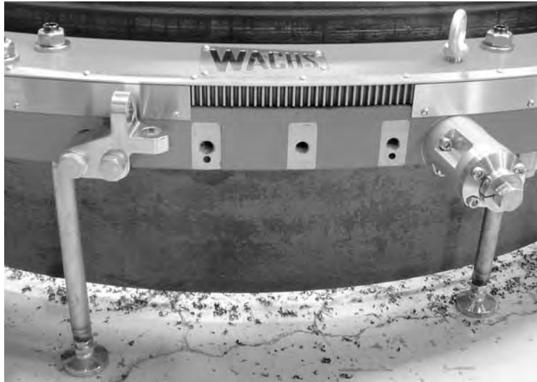
Figure 3-33. The photo shows the drive mounting location on the LDSF frame. The three screws in the drive assembly go into the three holes on the frame.
