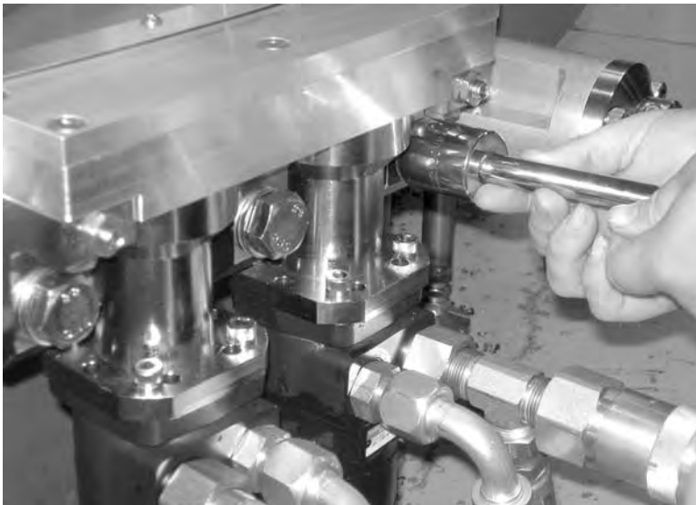
Figure 3-36. Tighten the screws holding the drive assembly.
