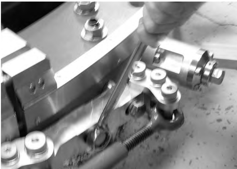
Figure 3-29. Tighten the two screws to secure the hinge to the stationary ring.
