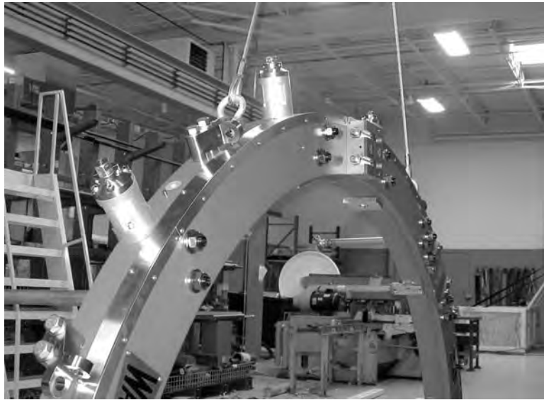
Figure 3-4. Lift the machine vertically as shown.
