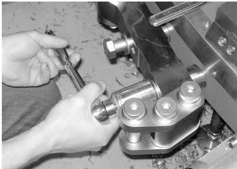
Figure 3-16. Insert and tighten the screws holding the hinge.
