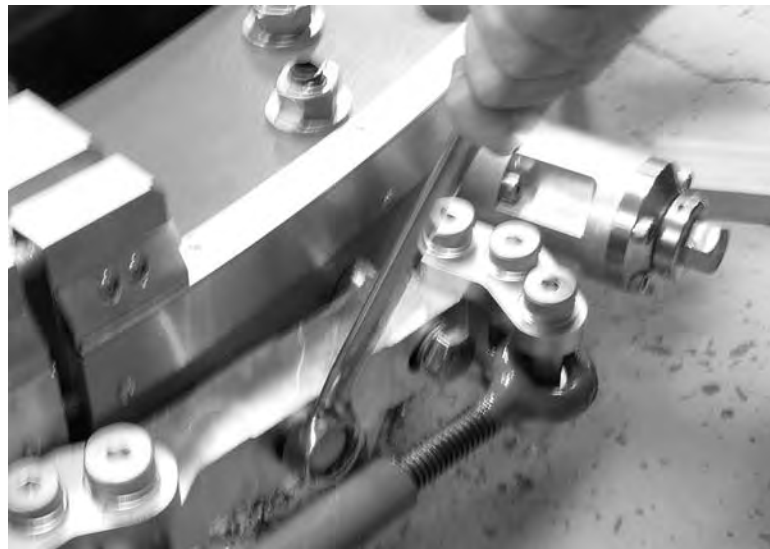
Figure 3-24. Tighten the two screws to secure the hinge to the stationary ring.
