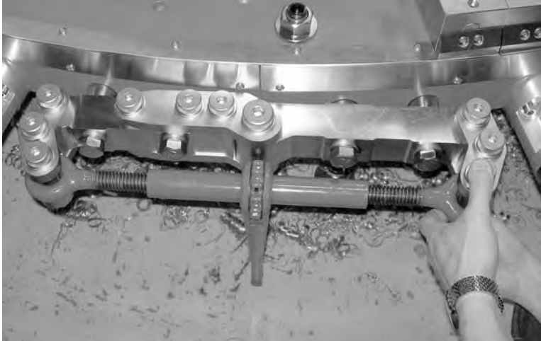
Figure 3-17. Mount the jack using the pins at the ends of the hinge.
