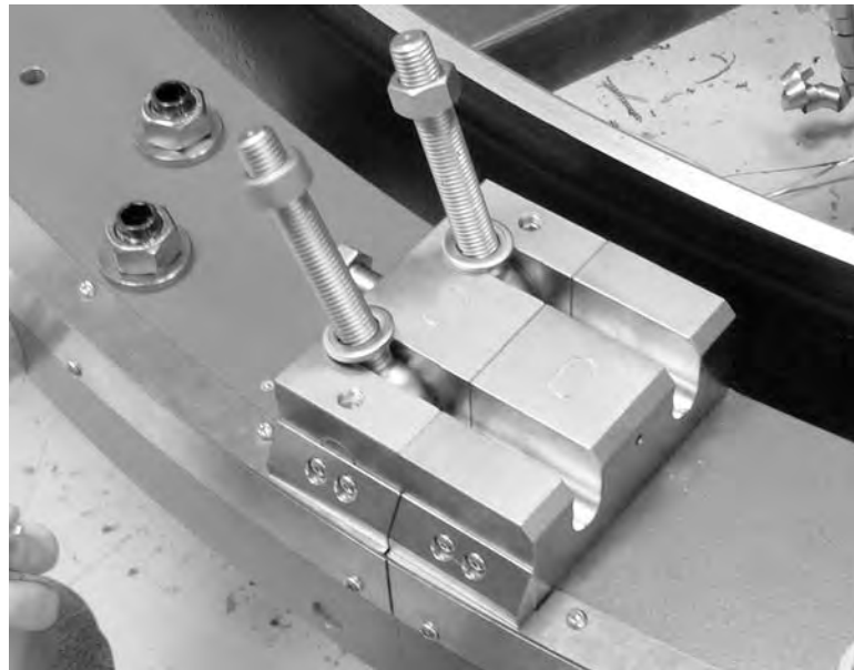
Figure 3-21. Loosen the nuts on the latch bolts (stationary ring, top photo, and rotating ring, bottom photo) and swing them out of the slots.
