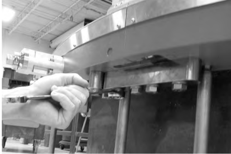
Figure 3-30. Attach the support block at the joint and tighten the 4 screws.
