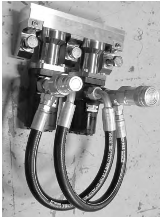
Figure 3-34. The photo shows the hydraulic drive assembly.
