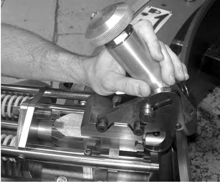
Figure 3-48. Loosen the pivot screw to set the counterbore slide angle.
