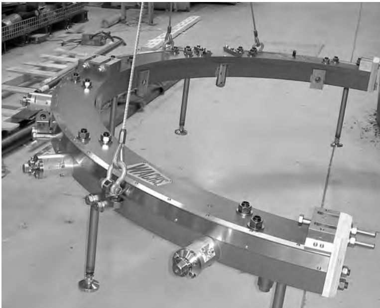
Figure 3-3. Lift the machine horizontally as shown.
