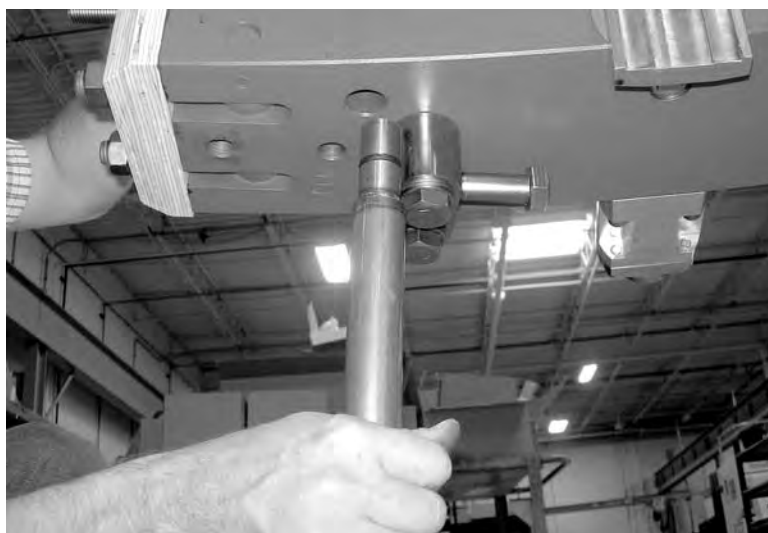
Figure 3-5. Insert the stand legs into the bottom of the stationary ring.
