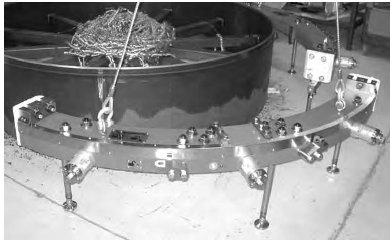
Figure 3-1. To lift an individual section, attach the rig to the lift eyes on top of the machine.
