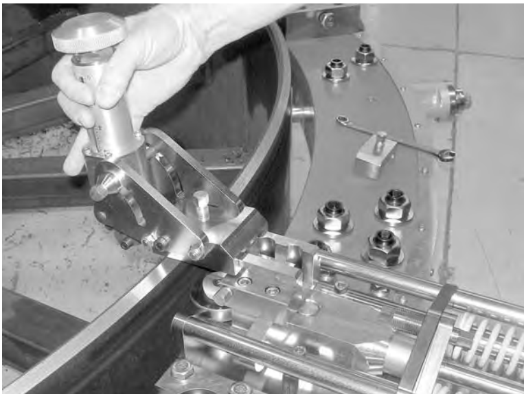
Figure 3-49. Mount the counterbore slide in the tool holder on the LDSF slide.
