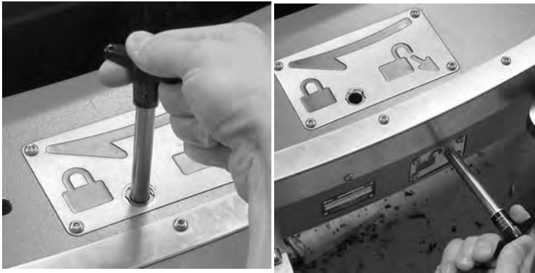
Figure 3-46. Remove the frame locking pins and put them in the parking holes in the stationary frame.
