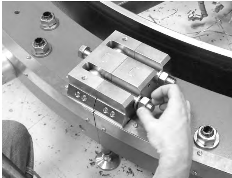
Figure 3-31. Swing the latch bolts into the slots and tighten the nuts.
