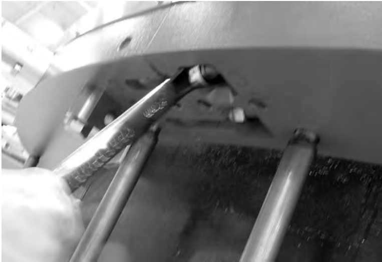
Figure 3-28. Tighten the nuts on the latch bolts.
