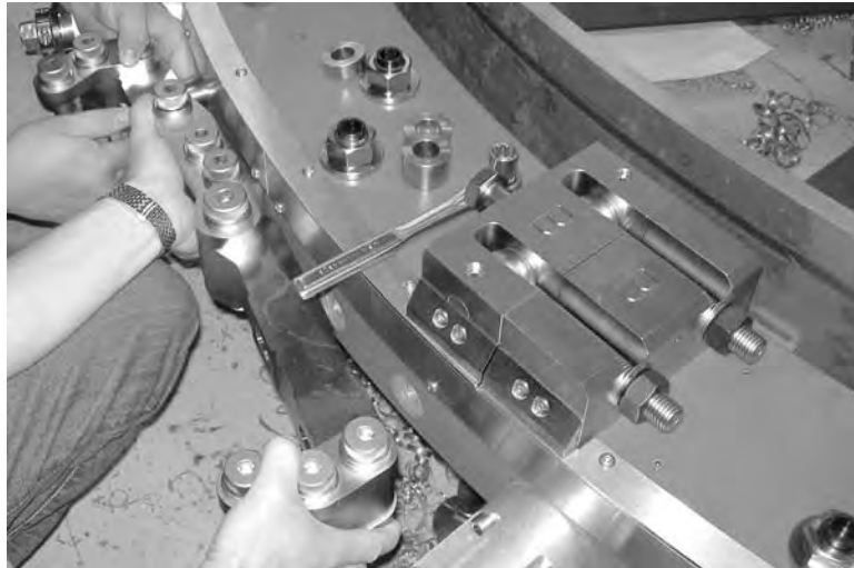
Figure 3-15. Attach the hinge to the stationary ring.
