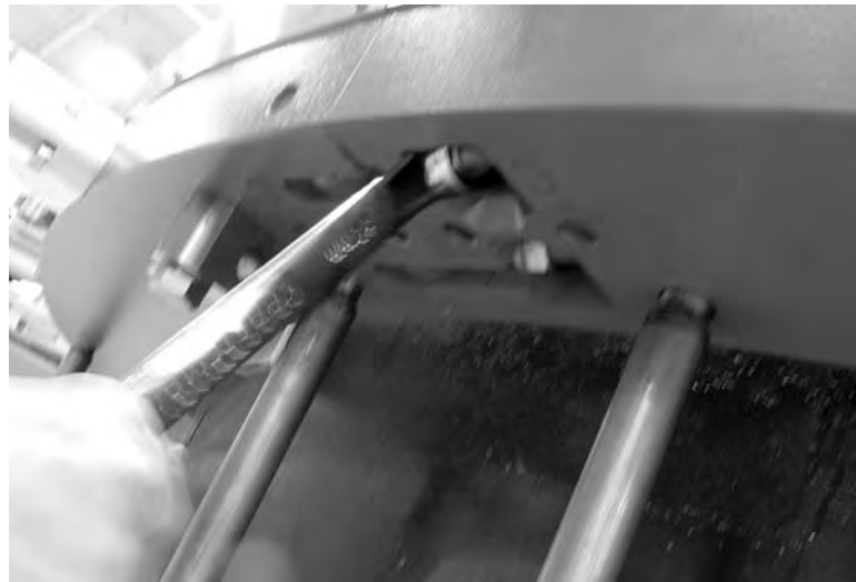
Figure 3-12. Tighten the nuts on the stationary ring latch bolts to secure the sections together.
