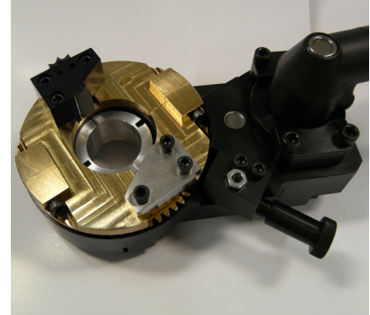
Figure 4 - Pneumatic UCSF (Ultra Compact Split Frame)
