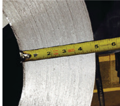
Figure 3 - Main Steam Outlet 4.78" (121.4mm) Heavy Wall
