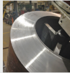
Finished Weld Prep Ready for Final Welding
