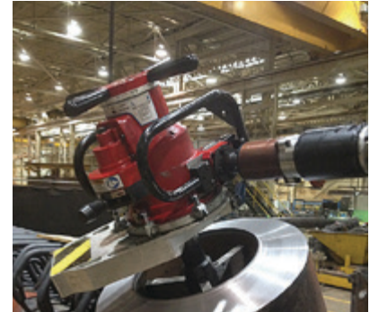
Figure 4 - Pneumatic EP 424 with Self Centering Mandrel
