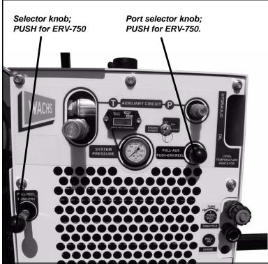
Figure 4-5. Push in both selector knobs to enable hydraulic flow to the ERV-750.
