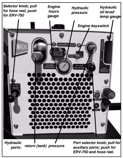
Figure 3-10. Front panel of the hydraulic power unit.
