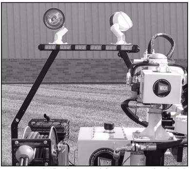
*Figure 3-17. The optional direction control and work light.*
