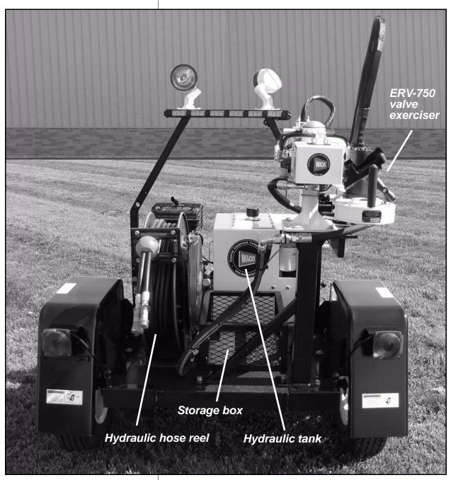
Figure 3-3. The rear view of the ERV Trailer System.
