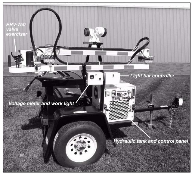
Figure 3-1. The right side of the ERV Trailer System.
