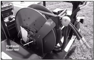
*Figure 3-16. The hydraulic hose reel is mounted at the rear of the trailer.*
