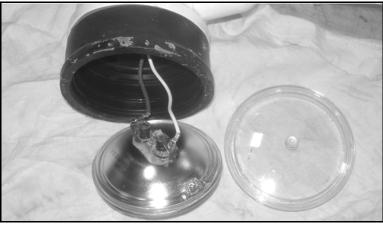
Figure 5-7. Pull the cover and bulb out of the rubber seal around the lamp housing.
