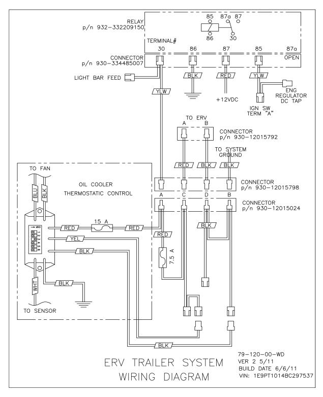
Figure 6-2. Wiring Diagram
