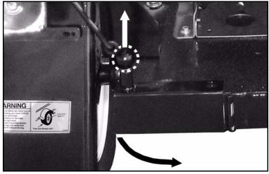
Figure 3-14. Access key storage by pulling the knob up and opening the cover toward the inside of the trailer.
