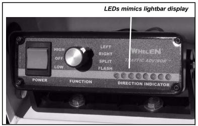
*Figure 4-13. Turn the function knob on the lightbar controller to select the display.*
