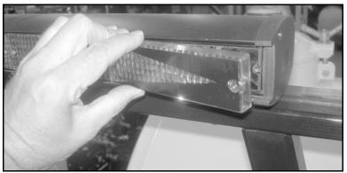
*Figure 5-5. Remove the two screws and pull the cover off the burned-out bulb.*
