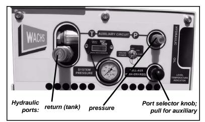
Figure 4-4. To use the auxiliary ports, connect hoses to the hydraulic ports and pull out the port selector knob.
