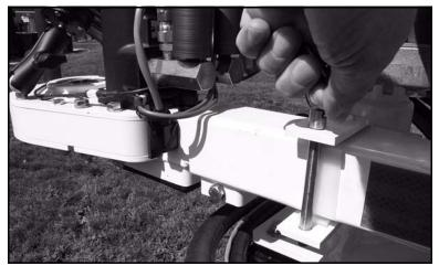
Figure 4-10. Pull the quick pin to release the ERV-750. Let the pin hang behind the arm when released to prevent entanglement of the lanyard.
