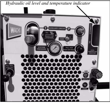
*Figure 5-1. Use the sight gauge to check oil level and temperature.*
