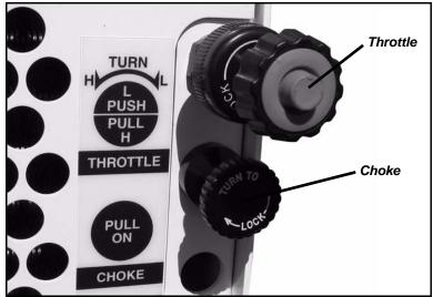
Figure 4-1. To start the engine, pull the throttle halfway out. If the engine is cold, also pull the choke out.
