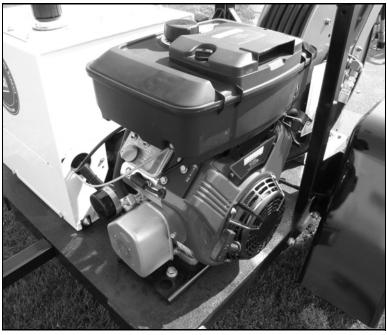
*Figure 3-8. The gasoline engine for the ERV Trailer System.*
