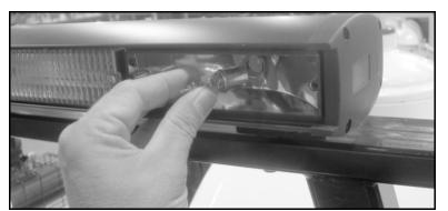
Figure 5-6. Remove the light bulb from the socket.
