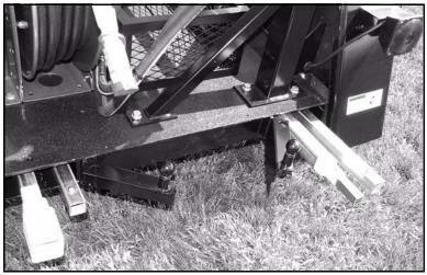
Figure 3-13. Additional key storage is located beneath the decking at the rear of the trailer.
