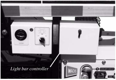
Figure 3-18. The light bar controller is housed in a water-tight enclosure above the hydraulic unit.
