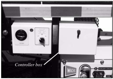
Figure 4-11. The light bar controller is inside a box on the right side of the trailer.
