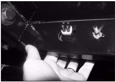
Figure 3-5. Route tongue connectors through frame.
