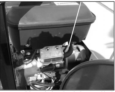
Figure 5-2. Use the dipstick to check engine oil level.
