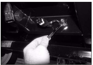
Figure 3-6. Attach ground wire to stud.
