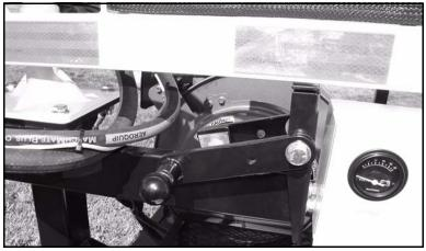
Figure 4-8. Secure the latch in the open position by releasing the knob under the lip of the arm.
