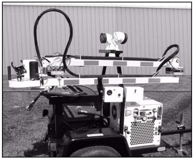
*Figure 3-12. The ERV-750 valve exerciser extends on a pivoting, telescoping arm.*
