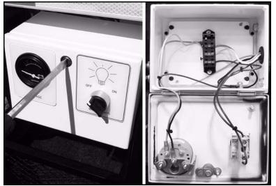
Figure 5-3. Insert a screwdriver to open the cover.
