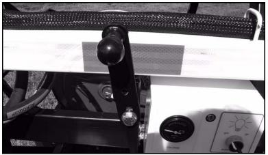
Figure 4-6. Release the latch by pulling the knob.
