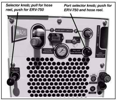
Figure 4-3. To use the ERV-750 or optional hose reel, first push in the port selector knob, then also either pull or push the selector knob labeled **PULL-REEL PUSH-ERV** as appropriate.
