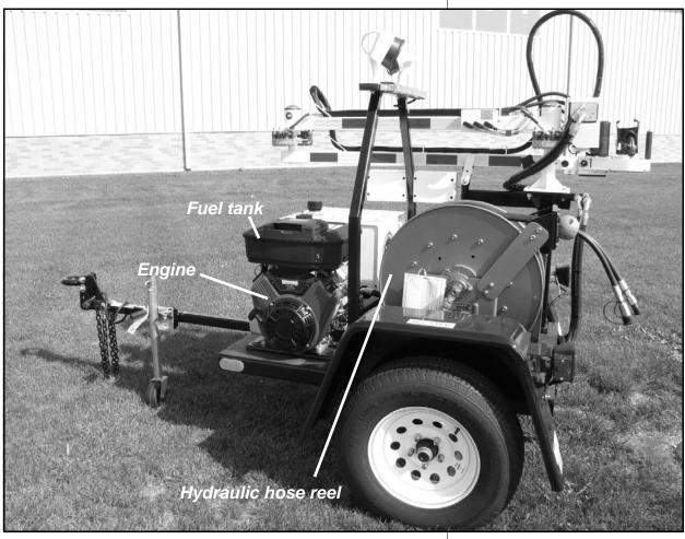
Figure 3-2. The left side of the ERV Trailer System.
