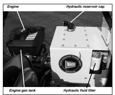
Figure 3-9. Components of the hydraulic power unit.
